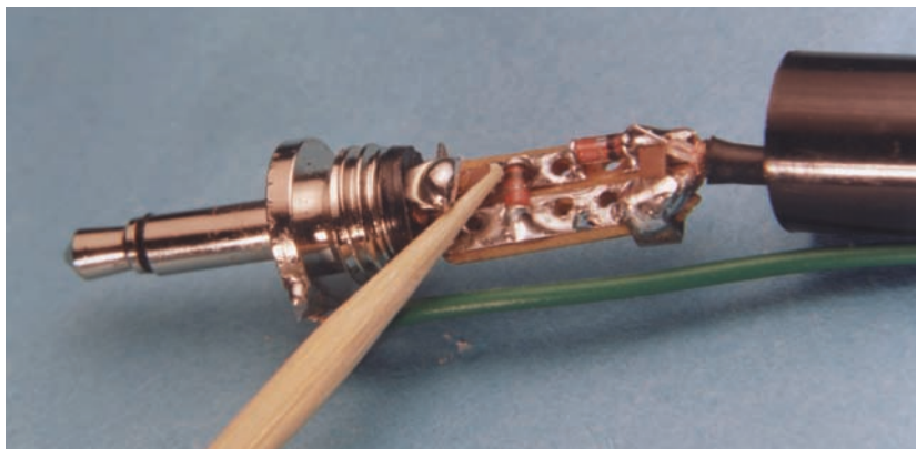
● Fig. 4: A probe built into a jack plug - a good indication of the small size of the project!
