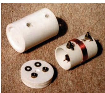
● Fig. 3: The construction of the traps, with the beehive trimmer inside the coils.
