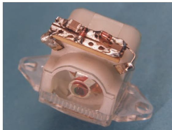
● Fig. 5: Probe detector mounted onto a (small) moving coil meter unit.
