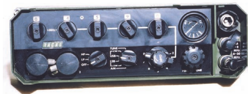
● Fig. 1: The miniature h.f. Manpack, PRM4031. The size can be judged from the BNC sockets on the right hand edge (see text).
