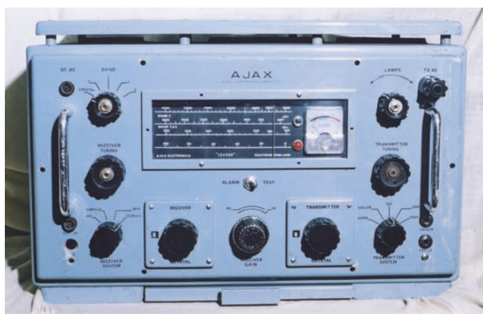
● Fig. 2: The Ajax Leader transmitter-receiver set. The receiver tuning is on the left. he transmitter tuning control is for p.a. tuning adjustment (see text).
