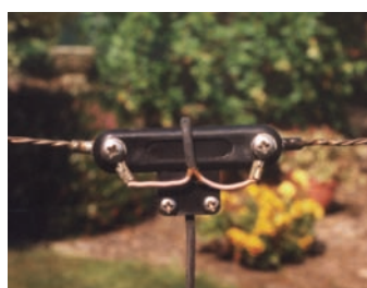
● Fig. 1: A commercial dipole antenna centre. Note that the 75Ω twin feeder loops over the top to reduce moisture ingress.
