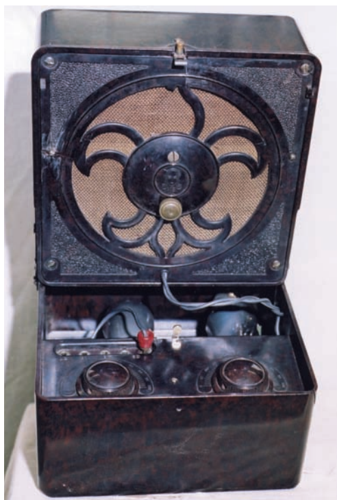
● Fig. 5: The KB Masterpiece t.r.f. vintage set, the two valves sit nicely inside the set with loudspeaker above (see text).
