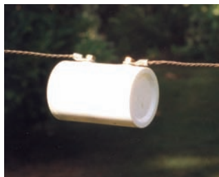
● Fig. 4: The trap inserted into the dipole. Make sure all connections are of good quality.
